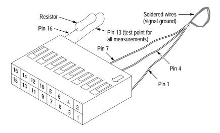
Figure 12: Threshold Fixture
