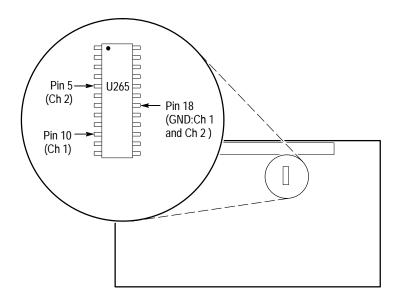
Figure 4: DAS 92E9 Expansion Slave Board Test Point Locations
