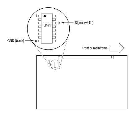
Figure 2: Controller Board 100 MHz Time Base Clock Test Point Locations (DAS 9219/9220 Mainframes)
