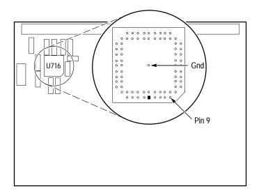
Figure 5: 92A16 Test Point Locations (back of board)
