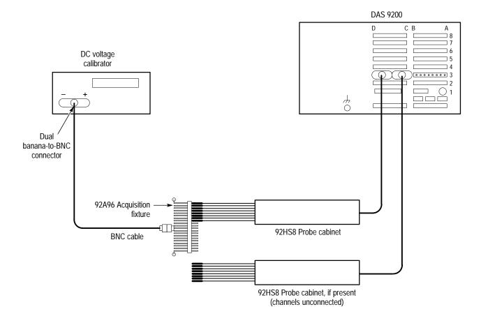
Figure 8: 92HS8 Probe Cabinet Data Threshold Accuracy Equipment Setup
